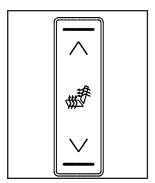
Your vehicle may have heated front seats. The buttons are located on the climate control panel.
